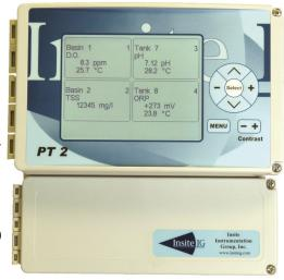
The backlit display can be programmed to show one, two, four, eight, or sixteen sensor readings continuously. If only one channel is displayed a trend graph of the last twenty four hours for that sensor will also be displayed. All sensor status and readings can be sent to the SCADA system or to a PLC via the two wire RS485 ModBus output.
