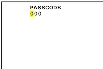
Use the “ARROW” keys to enter the first digit of the passcode, then press the “ENTER” key to proceed to the next digit. Repeat until all three passcode digits are entered.
