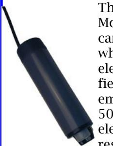
The Model 50 Electrode Holder with Model 51 replaceable pH Electrode cartridge comprise the pH sensor, which incorporates embedded electronics, custom geometry, and a field proven cartridge. The embedded electronics in the Model 50 Holder includes a built-in electrically isolated preamp, which results in reliable digital
